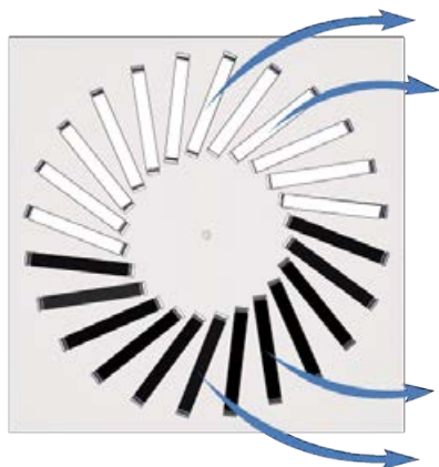
Setting of the air control elements
