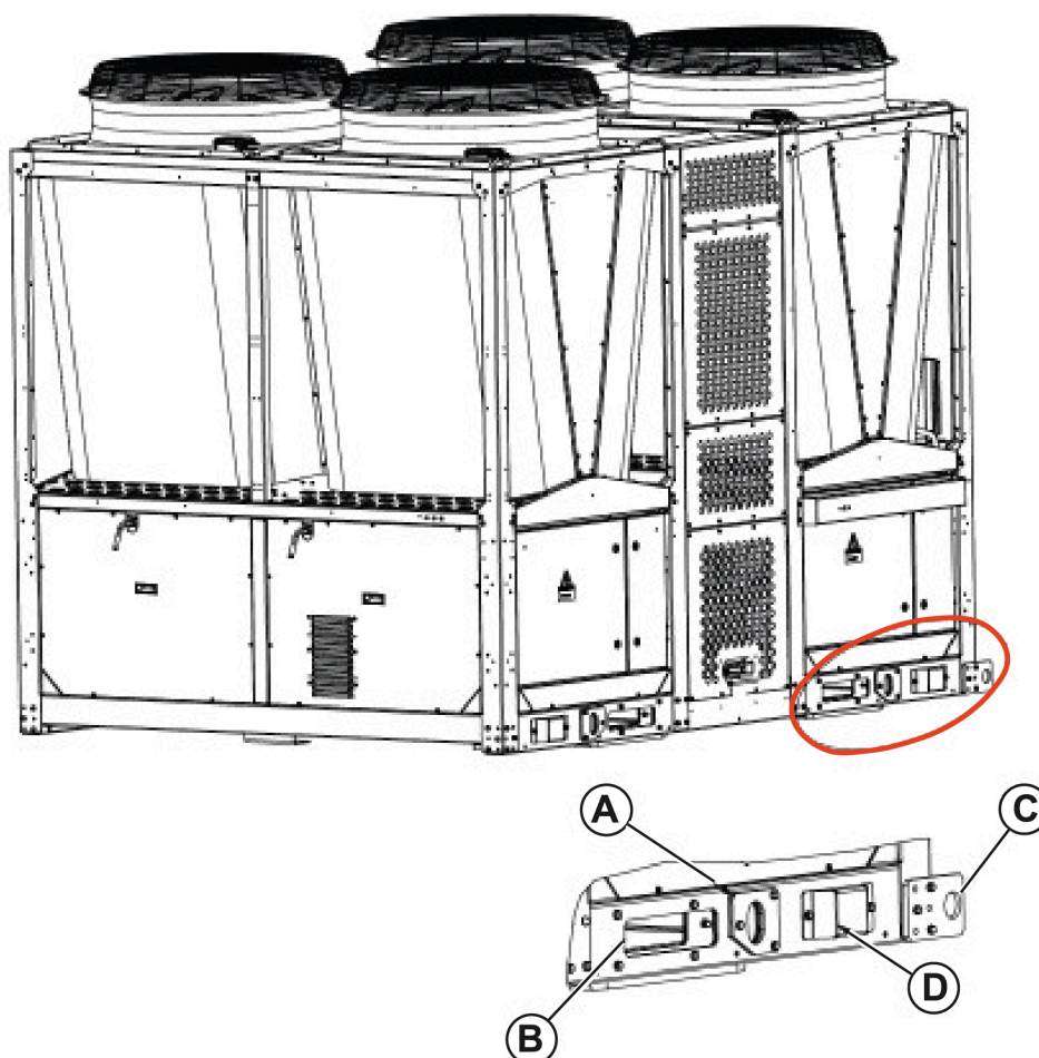
Figure 28: YMAE 0230 and 0260 rigging holes and fork lifting slots
